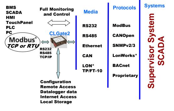
Modbus master (Client) Gateway configuration for integration of Modbus devices into other control systems (SNMP, Modbus, BACnet, etc)
