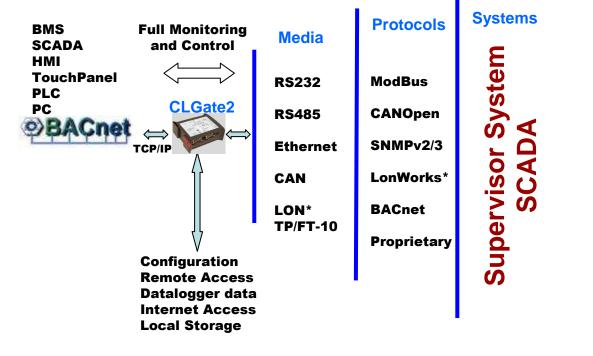
BACnet/IP Client Gateway configuration for integration of BACnet/IP devices into other control systems (KNX, Modbus, etc)
