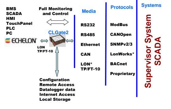
LonWorks master (Client) Gateway configuration for integration of LON devices or systems into other control systems (SNMP, Modbus, BACnet, etc)
