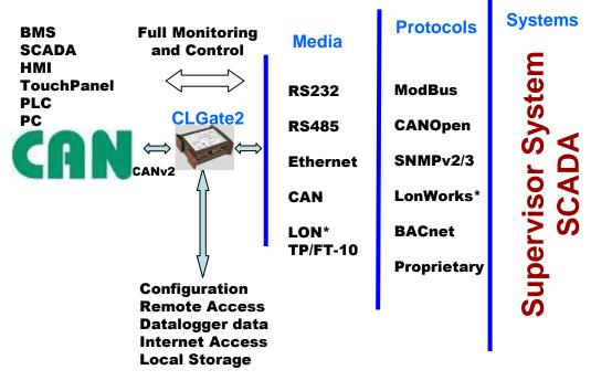
CANbus master (Client) Gateway configuration for integration of CAN devices into other control systems (SNMP, Modbus, BACnet, etc)
